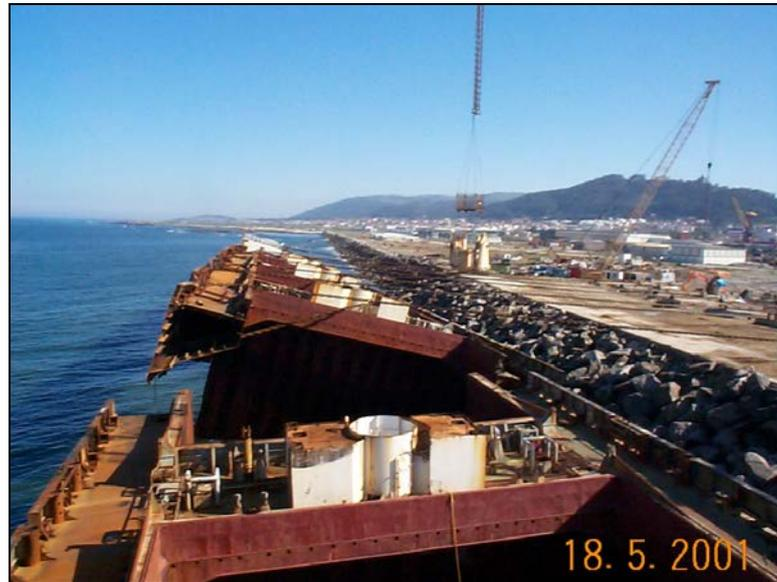
*Figure 8: Fore Part of the Wreck during early stages of Parbuckle operation*
