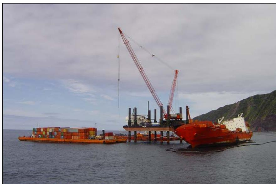
*Figure 6: Jack-up barge removing cargo from the wreck*
